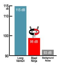
Blast Ninja™ reduces nozzle air exit velocity while maintaining particle velocity – therefore reducing noise production at the source while maintaining blasting production. Oceanit performed many years of extensive fluid dynamic modeling, lab analysis, field trials, and rigorous operator testing in various conditions to arrive at the final Blast Ninja™ product.
