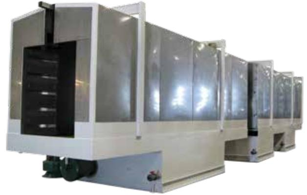
Our RTT skilled engineers will design a conveyor pass-through system specific to your needs, taking into consideration the size of the parts and the time allotted for the parts to pass through the washer.
