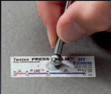
For use with Testex™ Press-O-Film™ Replica Tape
