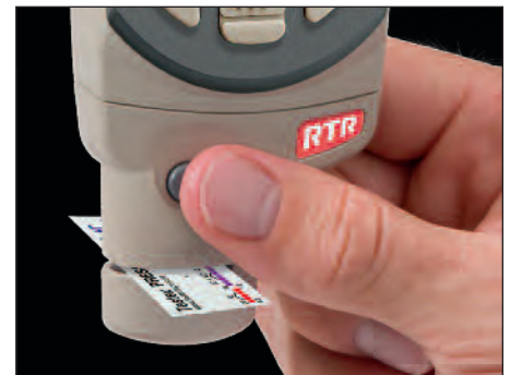
Align probe arrows with tape positioning dots
