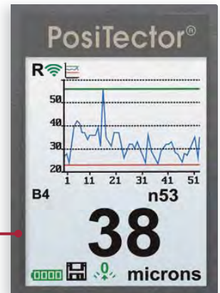
Advanced Model display shown in Memory mode with real-time graphing
