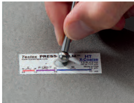
Stainless Steel Burnishing Tool ensures consistency
