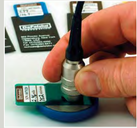
Steel and aluminum zero plates are available
